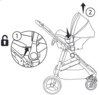
**2b.** Lift lever both sides of the adaptors to remove the adaptors from the chassis.
