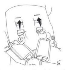
**3b.** Thread the waist strap retainers through the vertical slots in the seat unit backrest and thread the crotch strap retainer through the horiztonal slot at the centre of the seat unit.
