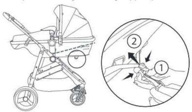
**4b.** Press buttons both sides of the seat connectors to adjust the seat unit recline. Ensure you hear a "click" as the seat engages at your desired position. **WARNING!** The seat unit is not suitable in pushchair mode for children under 6 months.
