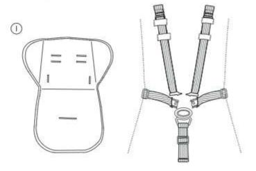
2. Thread the harness through the slots in the seat liner allocated for the waist, shoulder and crotch straps.
