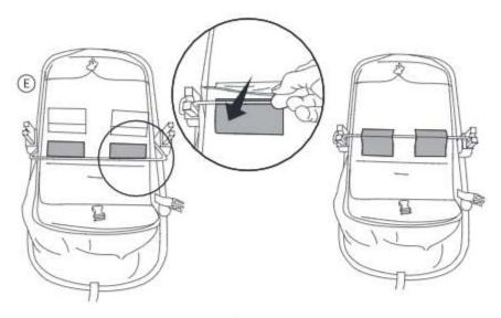
**2a.** Attach the seat unit to the chassis. Line up the seat connectors with the chassis housing and press downwards. Listen for a "click" to signal correct assembly.
