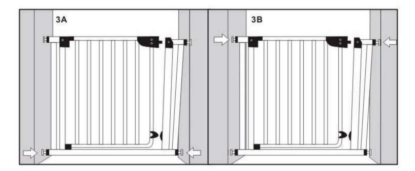
4. Tighten the Tension Knobs until the 2 Indicator Lines, located on the Upper Locking set and on the Right Upper Corner, align horizontally (4). Keep 1mm (0.04") gap between Upper Locking Set and Upper Right Corner (4).
