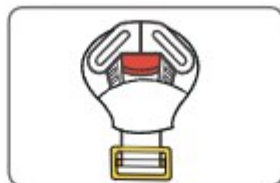
Insert the removed left and right buckle bolts into the buckle, and keep it in the buckle pad to avoid loss.
