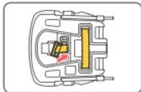
Slide the metal plate which is used to fasten the harness buckle to the seat shell down on its edge through the strap slot, remove the shoulder strap from the seat and keep it well.
