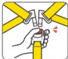
Release the 5-point buckle, change to Group II
