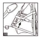
Press brake tab down to lock wheel or lift brake tab up to release wheel. See figure 11.
