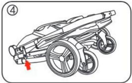
Follow the picture 3, press down the handle at the same time Follow the picture 4, finally lock the hook on the side.
