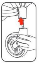
Lift the front wheel (As Shown in Figure). The opens of two front wheel bases are aligned to do the front foot, then hear the "click", which means that it has been in place. Press the detachable button in bottom of the front wheel and at the same time set aside the front wheels, you can detach.
