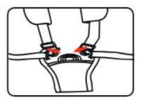
Follow the left picture: Press down the button to open the safety buckle. Follow the right picture: Insert the buckle to the socket, when hear click sound, then it's locked.
